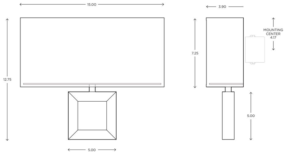
This fixture mounts independently from diffuser/backplate. The outlet box is located behind the diffuser.
